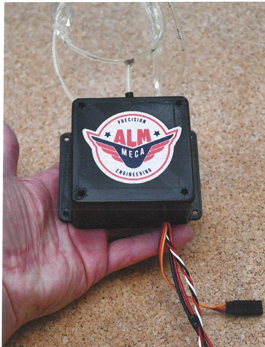
The combined Pump/ECU/Valve unit is quite large, but ALM-Meca will offer alternative designs of this to suit different models/installations.
