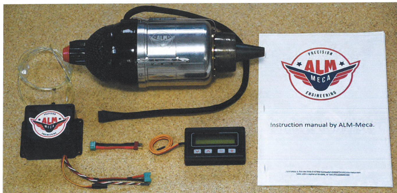
The A180 package has a minimal parts count as many components are installed within the combined Pump/ECU/Valve block.
