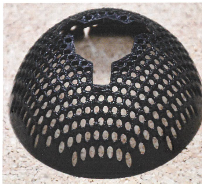
This neat 3D printed FOD guard is supplied with the turbine.
