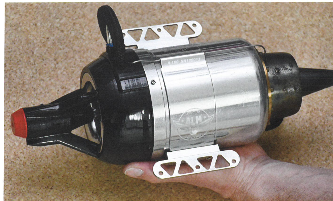
View of the turbine itself, note the substantial machined alloy mounts and the well protected main electronics cable from the engine.
